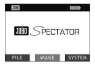
On the start up screen, you can use the buttons  $\blacktriangleleft$  or  $\blacktriangleright$  to select one of the three modes; FILE, IMAGE or SYSTEM mode. To confirm press the  $\Box$  button. The selected mode is highlighted in red.
